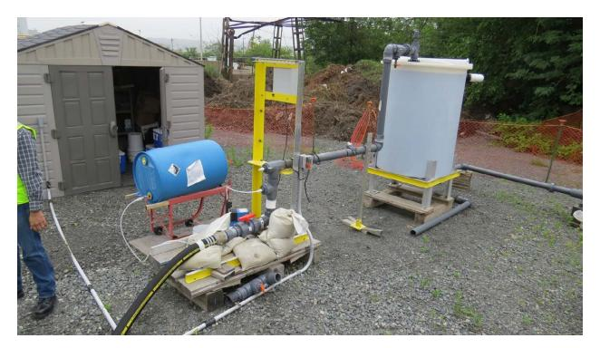
Figure 1. Peracetic acid Peragreen INJEXX system on project site
