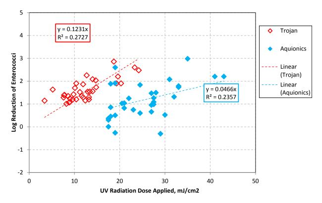
Figure 12. UV dose applied vs log reduction of Enterococci
