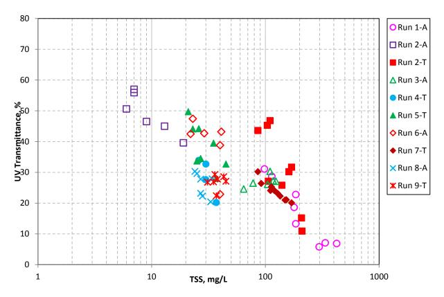
Figure 14. Effect of TSS on UV transmittance – grouped by Test Run
