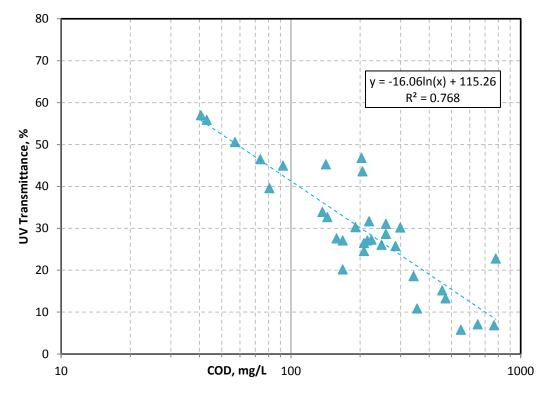
Figure 16. Effect of COD on UV transmittance
