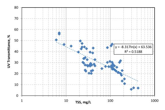
Figure 13. Effect of TSS on UV transmittance
