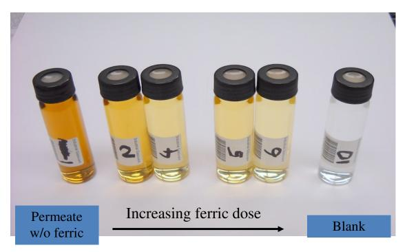
Figure 4. Effect of Ferric Addition on Permeate Color.
