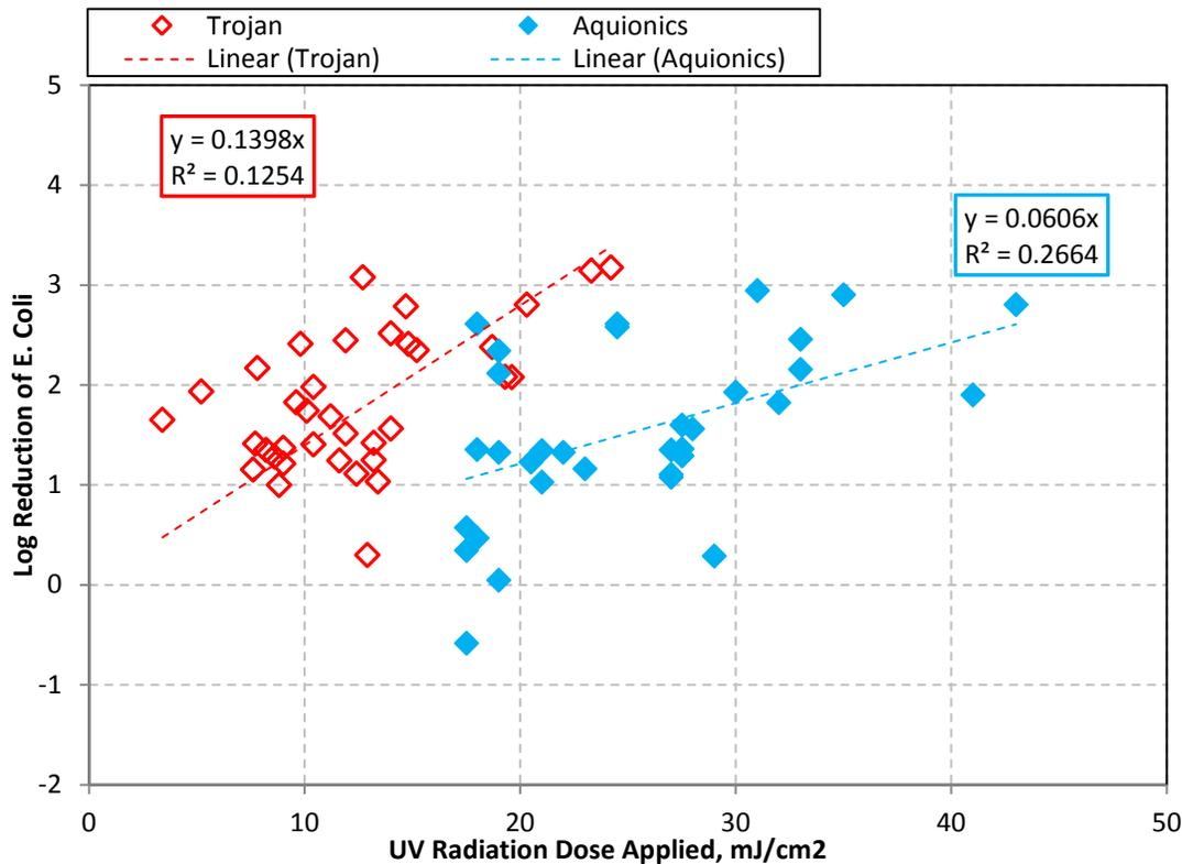
Figure 10. UV dose applied vs log reduction of E. Coli
