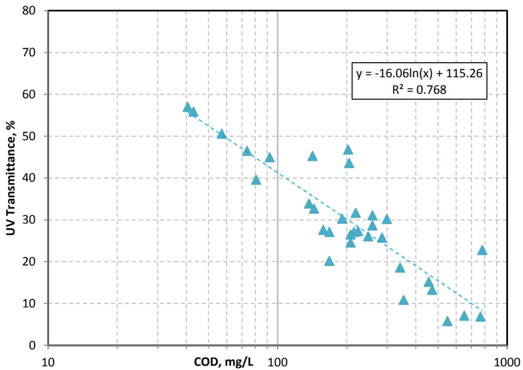
**Figure 16. Effect of COD on UV transmittance**
