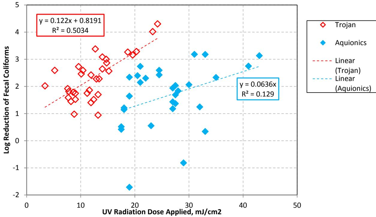
Figure 11. UV dose applied vs log reduction of fecal coliforms
