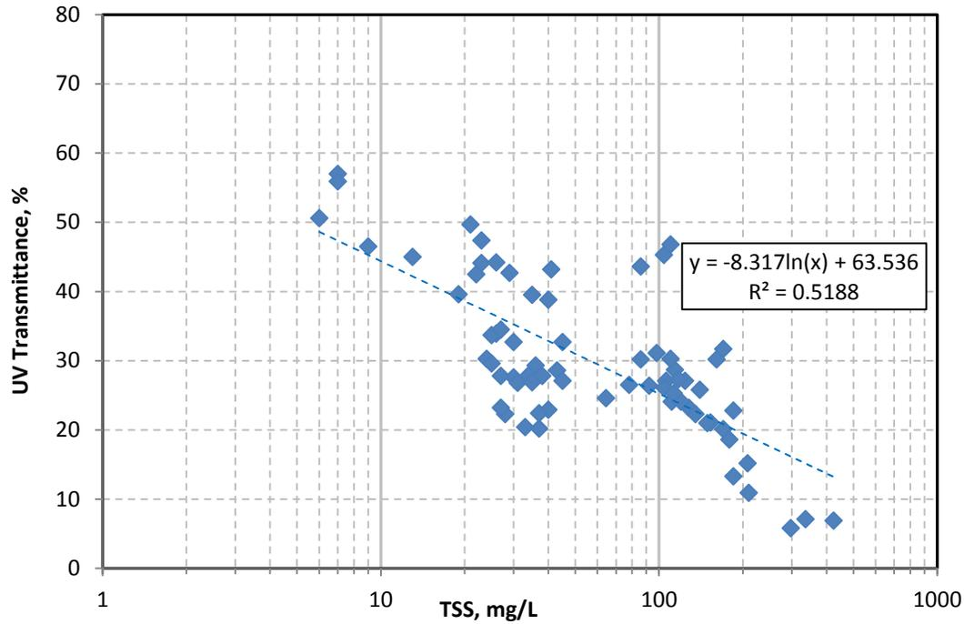
**Figure 13. Effect of TSS on UV transmittance**
