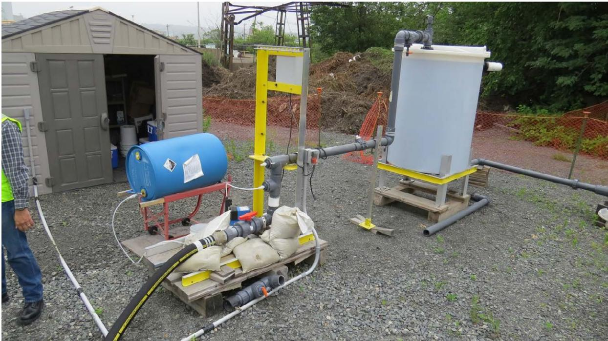
**Figure 1. Peracetic acid PeraGreen INJEXX system on project site**
