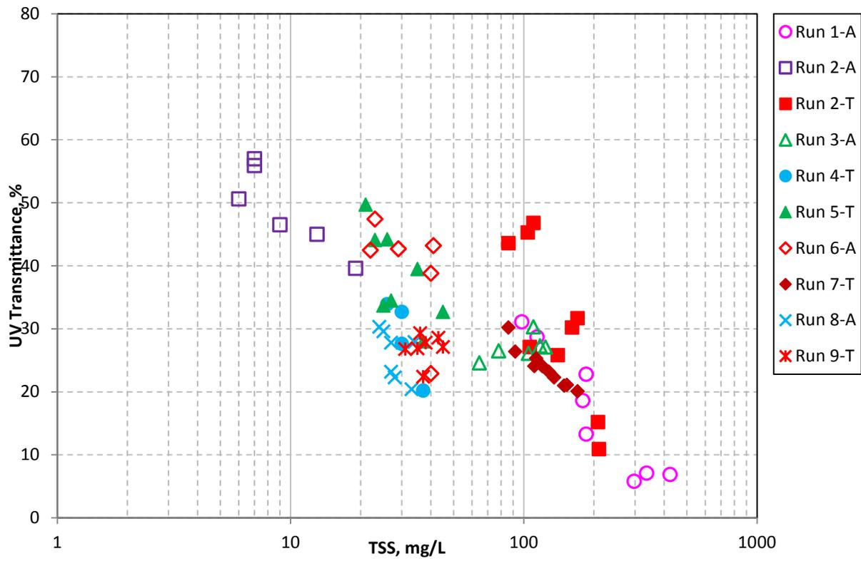
**Figure 14. Effect of TSS on UV transmittance – grouped by Test Run**
