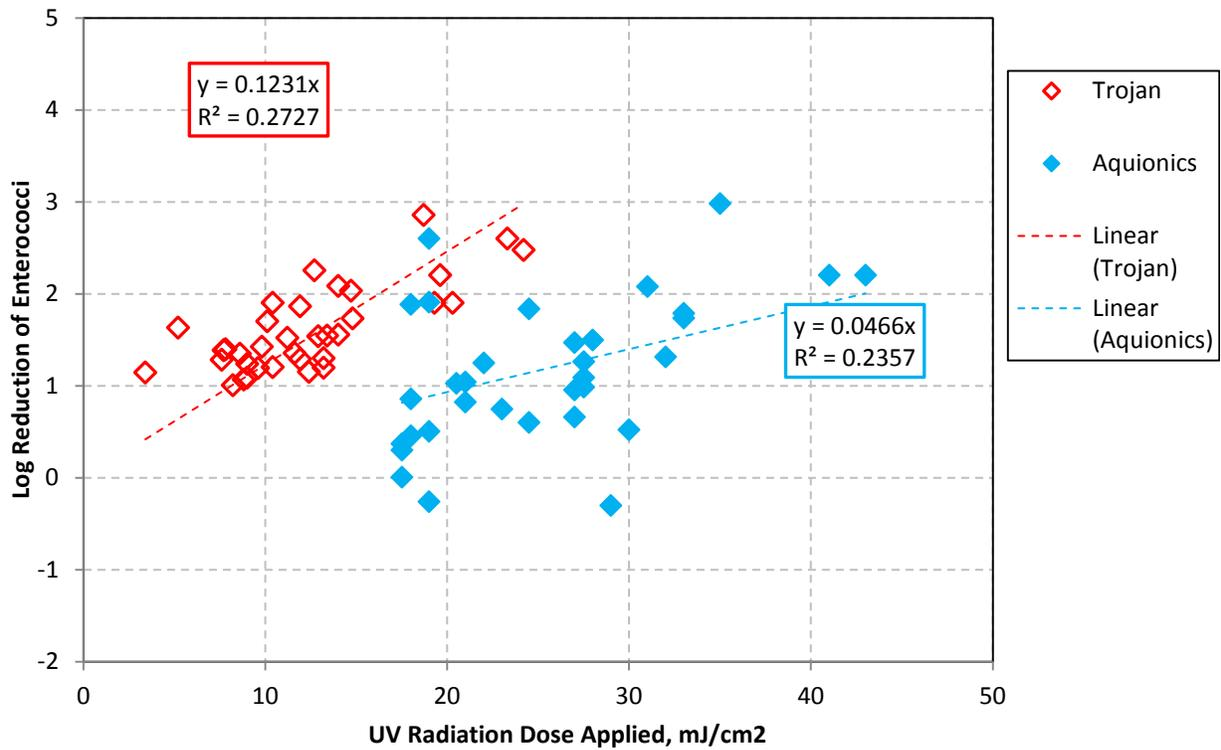
Figure 12. UV dose applied vs log reduction of Enterococci
