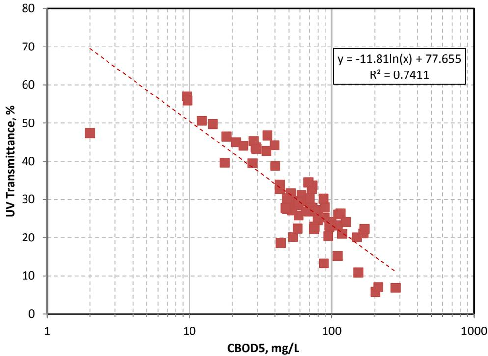
**Figure 15. Effect of CBOD<sub>5</sub> on UV transmittance**
