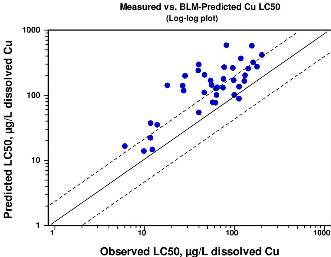
**Figure 3. Log-log plot of measured versus BLM-predicted Cu LC<sub>50</sub> values for stream samples collected in Michigan's Upper Peninsula. Solid line represents the theoretical line of equality; dashed lines indicate when BLM-predicted values are within a factor of two.**
