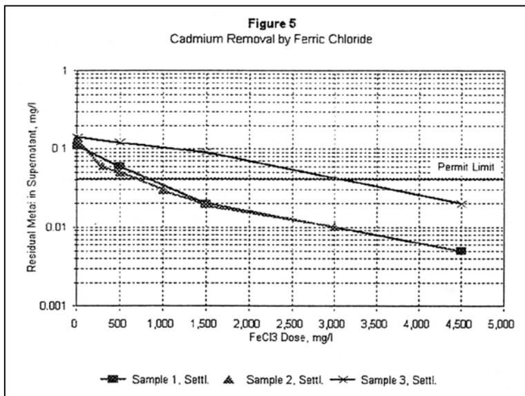
As in the previous projects, the chemical of last resort, which was ferric chloride, was used. Following ferric chloride addition, the pH was adjusted to 7.5 (in accordance with information in Table 1), sample flocculated for 30 minutes, settled and heavy metals analyzed, in filtered and unfiltered supernatants.
