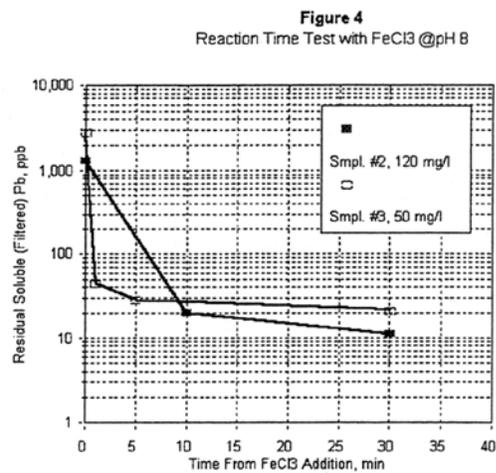
Based on Figures 2 and 3, the effective doses to meet the target 0.10mg/l ppb level in all samples tested, were 50 and 30mg/l for FeCl<sub>3</sub> and PQA respectively. However, due to much higher unit cost of the proprietary PQA, ferric chloride was recommended by more than a 2:1 ratio, as the more economical alternative. The required dose of ferric chloride was much higher than recommended by Macchi (1993) in his lead battery wastewater application, where ferric dose was based on Fe/Pb ratio.
